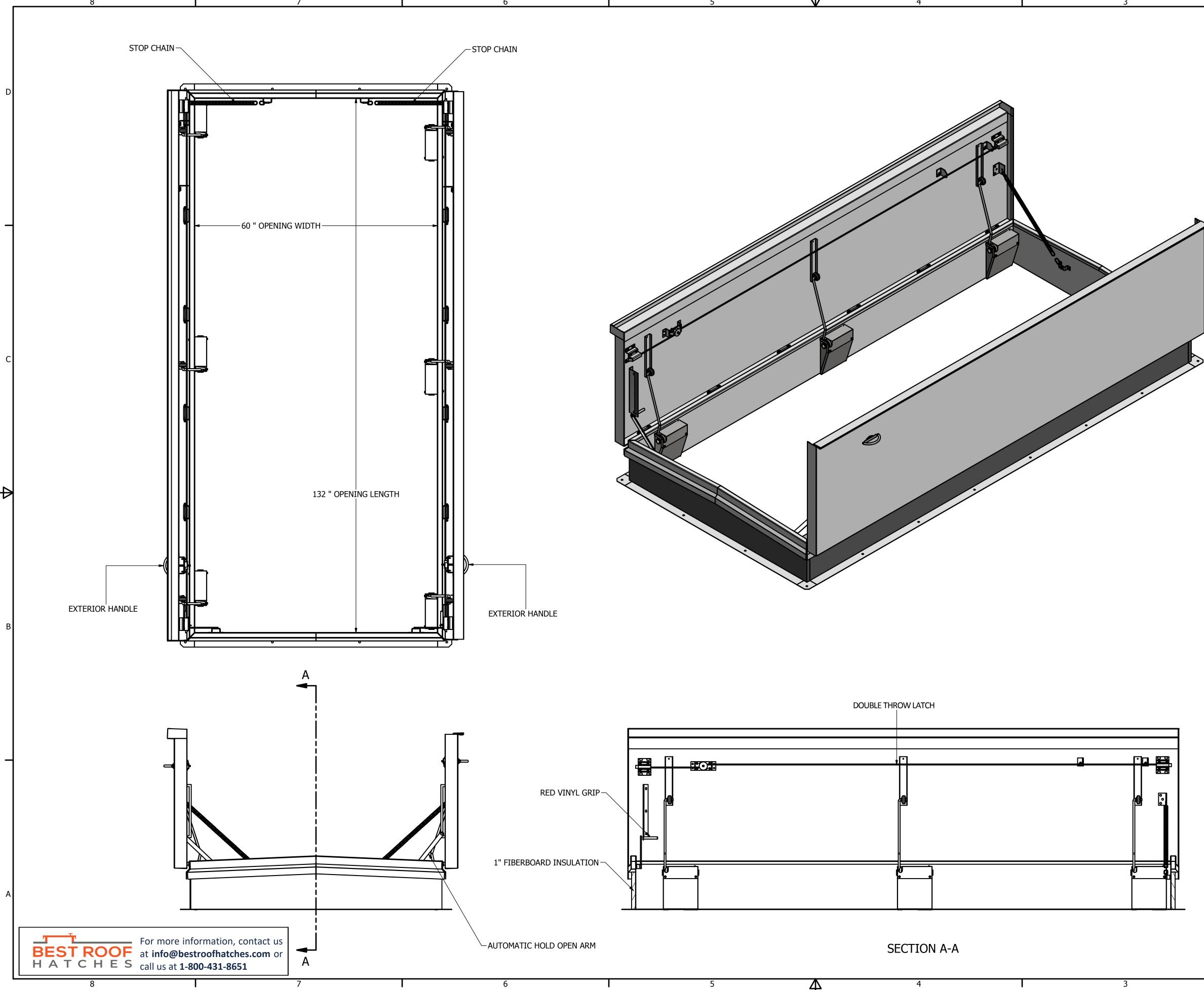
NOTES: SIZE: RB-5'0"X11'0" 1) 40psf COVER LIVE LOAD RATING 2) HATCH PAINTED WHITE 3) MATERIALS: 14ga GALVANIZED, COVER 14ga GALVANIZED, CURB 14ga GALVANIZED, COUNTER FLASHING 22ga GALVANIZED, COVER LINER
