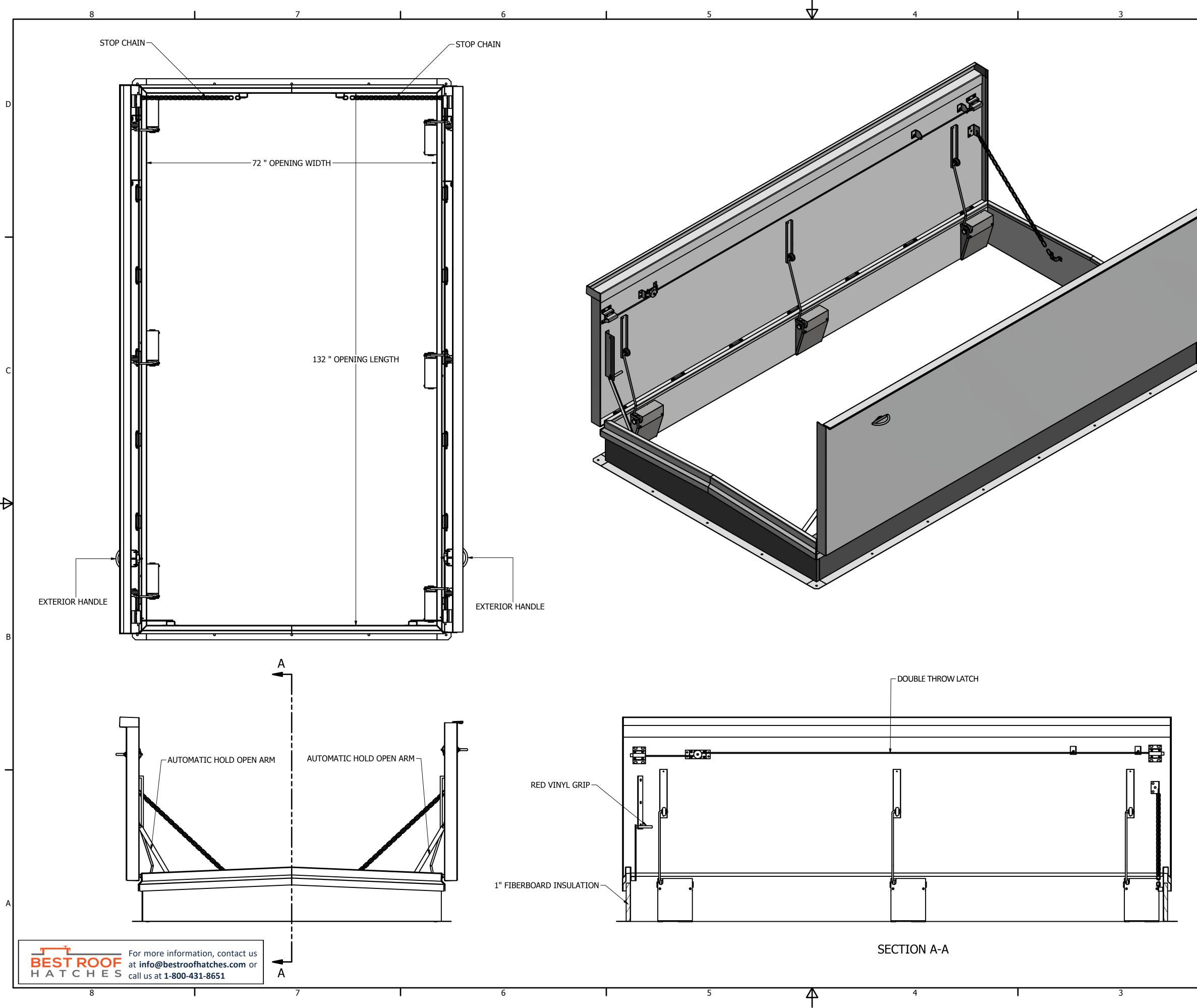
NOTES: SIZE: RC-6'0"X11'0" 1) 40psf COVER LIVE LOAD RATING 2) MILL FINISH 3) MATERIALS: .090 ALUMINUM, COVER 14ga GALVANIZED, CURB 14ga GALVANIZED, COUNTER FLASHING .063 ALUMINUM, COVER LINER
